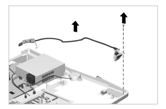
Figure 6-27. Removing the IrDA Board
